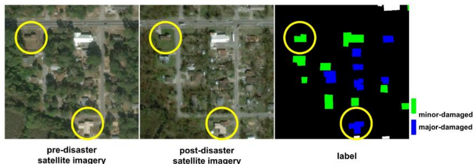
Figure 3. Examples of damage labels in the xDB dataset. The pre- and post-disaster images of minor damaged structures are nearly identical, yet they show substantial visual differences for major damaged buildings.
